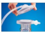
2. Attach inlet feedline tubing to the tapered inlet on the upper housing. Place upper housing onto housing base to securely seal the membrane.
